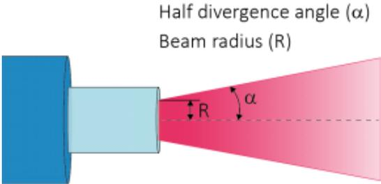
*The BPP value of the laser beam delivered from a fiber optic cable is given as the product of fiber core radius and output divergence angle (half angle). Smaller fiber core radius and/or smaller output divergence angle give a better beam quality (lower BPP-value).*
