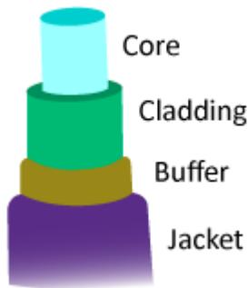
In an optical fiber the part with the higher reflective index is called the “core” and the material, with lower reflective index, surrounding the core, is called the “cladding”. For high power applications, only fibers with a core made of pure fused silica are used. The most common design surrounds the core with a cladding made of doped silica. Outside the cladding, there are at least two more layers to protect the fiber and make it flexible—the “buffer” and the “jacket”.
