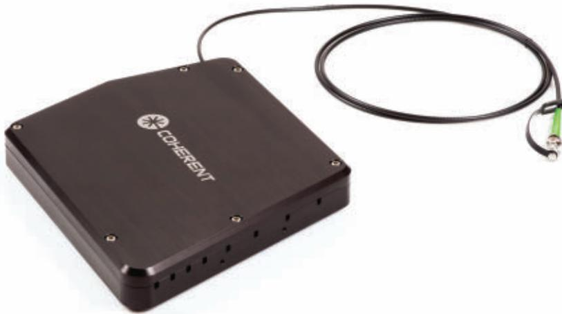
**Figure 4.** The OBIS Galaxy optical bus uses eight wavelength-dedicated plug-and-play input sockets to combine multiple lasers in a single output fiber. Courtesy of Coherent.
