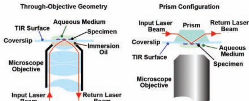
**Figure 1.** In TIRF microscopy, excitation light beyond the critical light is completely reflected. The evanescence of the light field at the refractive interface penetrates into the sample by about 100 nm, causing selective excitation of molecules and complexes adhered to this interface. TIRF microscopes are available with a choice of either through-objective excitation or prism excitation options.
