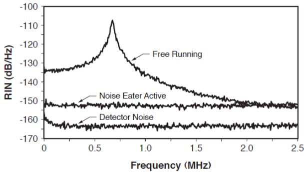
**Figure 6** Mephisto amplitude noise, expressed as RIN (Relative Intensity Noise) between 0 and 2.5 MHz. The Noise Eater circuit is effective in eliminating most of the pump diode current noise as well as the noise peak due to relaxation oscillations.
