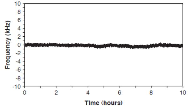
**Figure 5** Ten hour stability run of Coherent's Mephisto (1064 nm) locked with Iodine Frequency Stabilization option.
