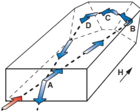
**Figure 2** In a NPRO the gain crystal forms a monolithic laser cavity, where the facet angles ensure high reflectivity through total internal reflection (TIR). The facets are arranged so that polarization rotation (due to TIR) in combination with an externally applied magnetic field preferentially supports unidirectional traveling wave laser operation.
