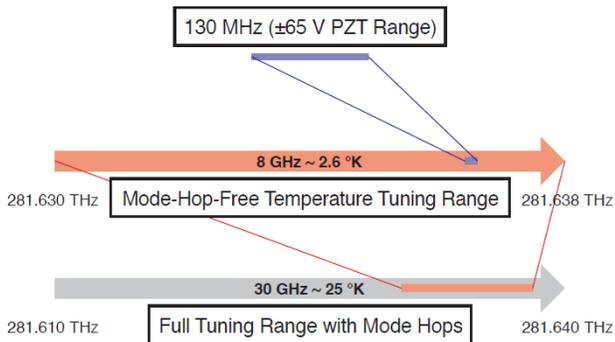
**Figure 4** Mephisto frequency tuning ranges with PZT and temperature controller.
