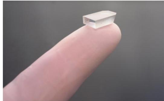
**Figure 1** Size scale of the NPRO crystal which lives in the heart of Coherent's Mephisto family of lasers.
