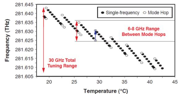
**Figure 3** The Mephisto output frequency as a function of crystal temperature. Mode -hops and regions where two modes can simultaneously oscillate are also indicated.
