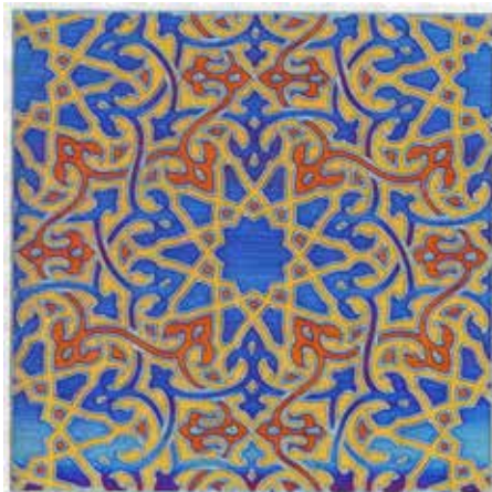
Figure 1: Vivid color marks with incredible detail can be created on metal samples such as this 25 mm x 25 mm sample using a Coherent picosecond laser).
