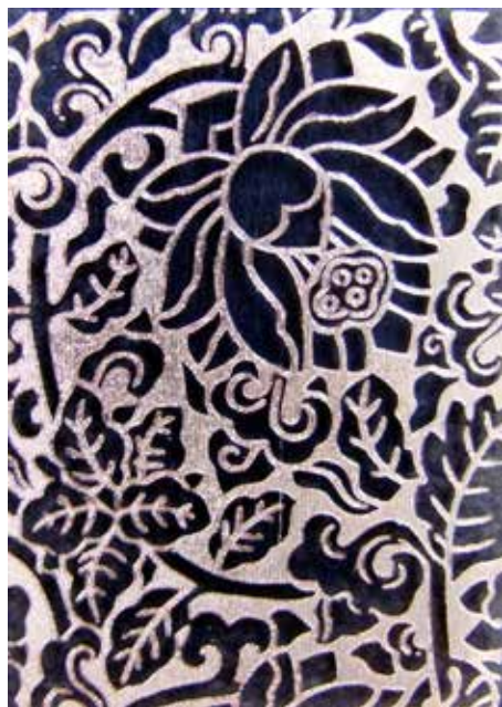
Figure 3: Another process enabled by picosecond lasers was used to create this metallic pattern (18 mm × 25 mm) in clear glass
