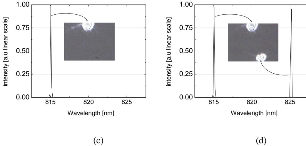
Fig. 4. (a) Extended wavelength tuning range self-aligned ECL based on multiplexed gratings. (b) Experimental demonstration of the concept with a two line VHG and a reflective mirror in place of the LCD. (c,d) experimental results: the two modes of the cavity corresponding to the two multiplexed gratings are simultaneously competing. The insert is an image of the secondary beams.
