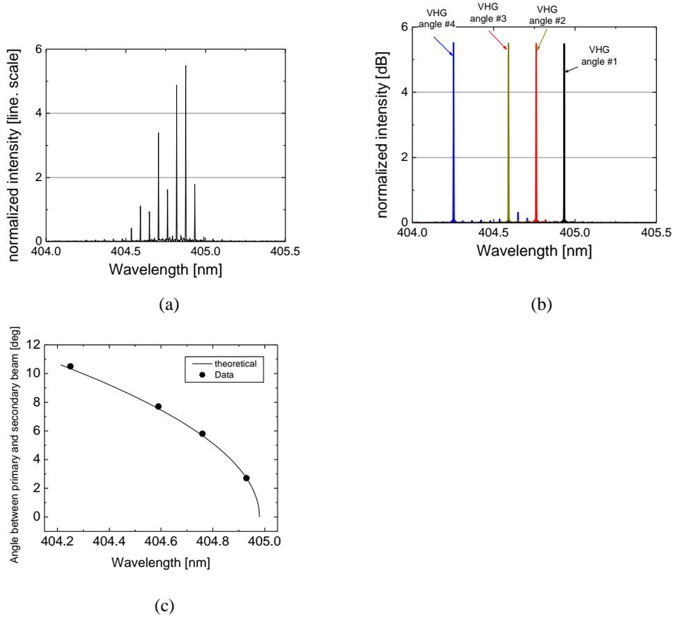
Fig. 3. (a) original diode spectrum of a 10 mW, blue-violet 405 nm laser diode (b) spectra of the ECL at different VHG angles. (c) angular wavelength tuning of the VHG in the plane of Fig. 2. Angles are measured between the output beam and the secondary beam (values are twice the rotation angle of the VHG)
