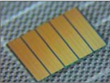
Figure 2. A Coherent | DILAS T-Bar chip contains five emitters, outputs about 50 W, and is 5 mm wide.
