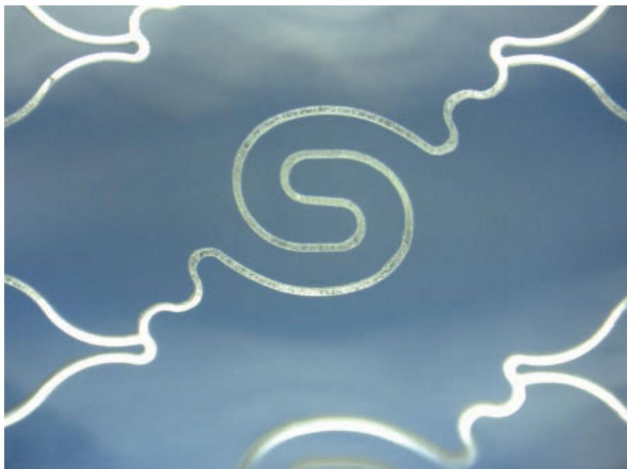
Stent with ultrafine structures fabricated with a Spirit industrial femtosecond laser. Strut widths and thicknesses are  $<50 \mu\text{m}$ . Courtesy of Spectra-Physics, a Newport Corp. brand.
