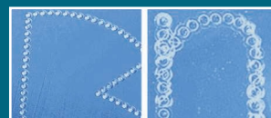
► Figure 2: Engravings in mineral glass using the 193 nm Excistar laser at a spot size of 40 μm (left image) and a q-switched pulsed CO 2 laser at a spot size of 120 μm. The CO 2 laser mark shows thermal effects due to the longer wavelength, including uncontrollable microcracking. ►
