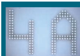
► Figure 4: Technical engraving of 80 µm diameter spots in transparent polymer material shows the superior quality obtained using the 193 nm excimer laser. The width of each spot is slightly larger than the width of a human hair. ►
