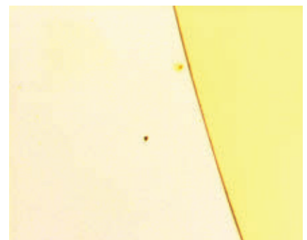
Figure 2. A CO laser with only 9 W of output power produced a clean, curved cut (6-mm radius circle) in thin glass (50- \mu\text{m} thick).
