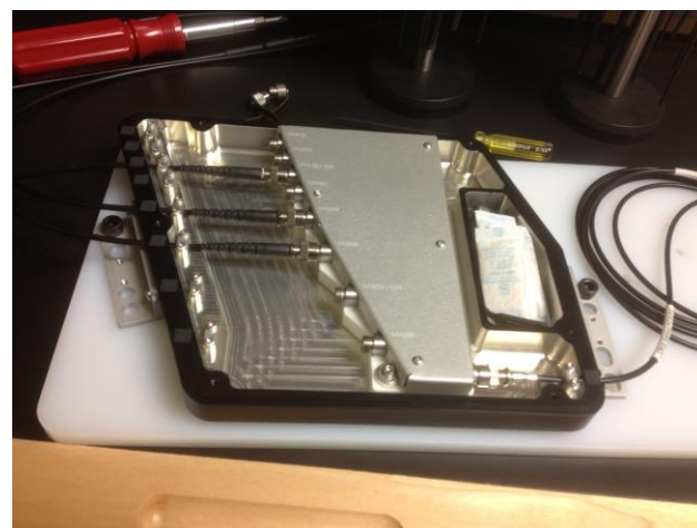
Figure 2 The OBIS Galaxy (shown with the top cover removed) allows plug & play combining of up to eight separate fiber coupled lasers into a single output fiber. Image courtesy Sam Lord.
