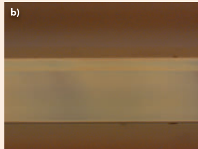
Cross-sections of 0.7mm-thick Corning CT24 glass, taken with a Nomarski differential interference contrast microscope. The piece cut with a CO 2 (~10 \mu m) laser (a) shows residual stress, while the cut produced with the CO (~5 \mu m) laser (b) is defect-free.
