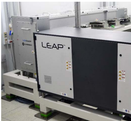
Figure 6. UVblade LLO system with LEAP excimer laser and line beam optics.
