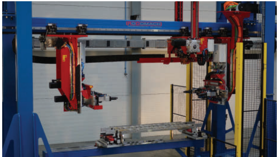
Figure 4. A system for automated welding of towel radiators. Courtesy of Coherent Inc.
