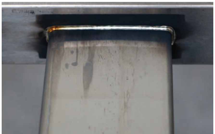
Figure 3. Detail of a weld seam produced by a fiber laser-based system. Courtesy of Coherent Inc.
