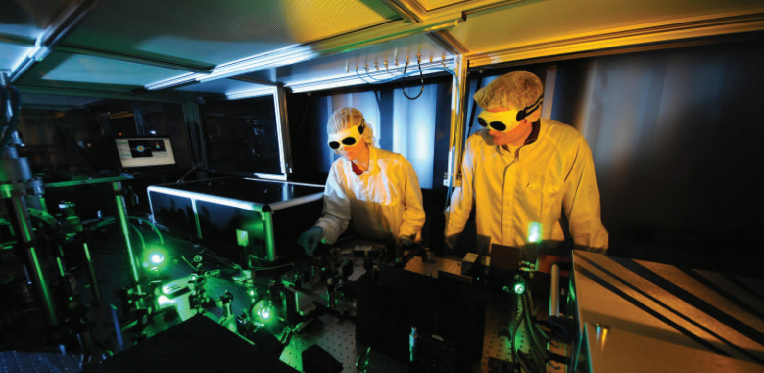
Doctoral students adjust the pump laser of a high-repetition rate optical parametric chirped pulse amplifier (OPCPA) at the Munich-Centre for Advanced Photonics (MAP).
