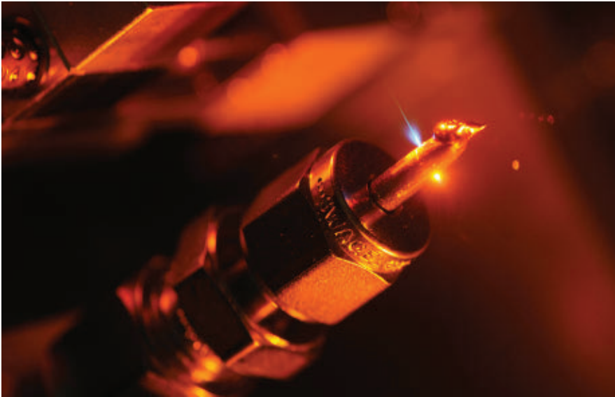
Gas-filled capillary used for the generation of attosecond light pulses in an attosecond beamline (AS-5).
