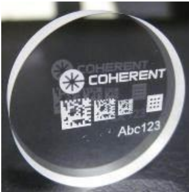
Picosecond lasers can be used to mark sapphire, which is difficult to mark by other means due to its extreme hardness
