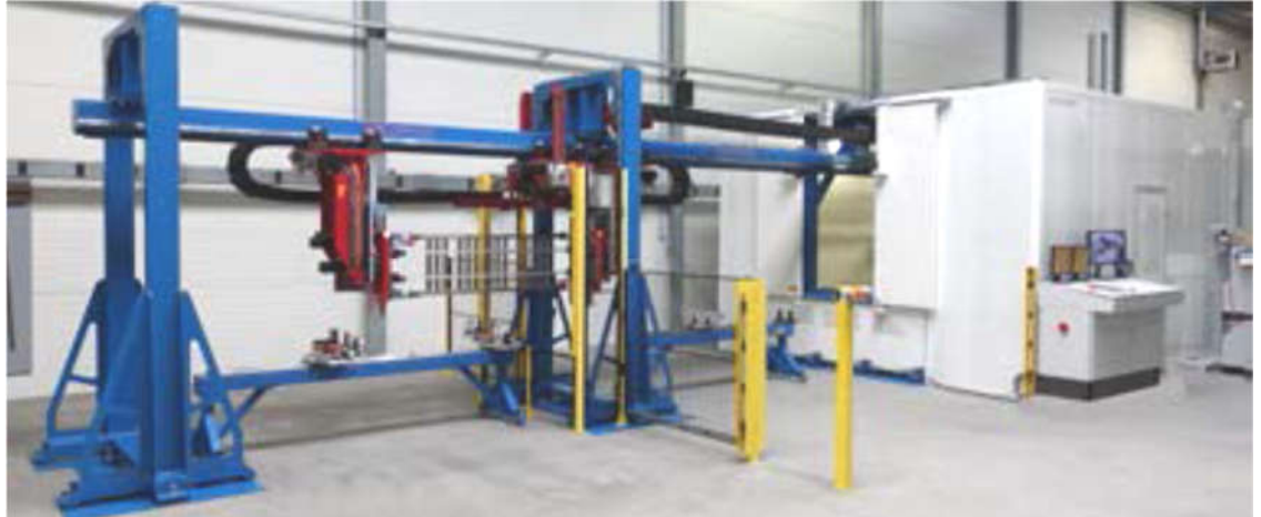
Figure 3: Complete system for automated welding of towel radiators.
