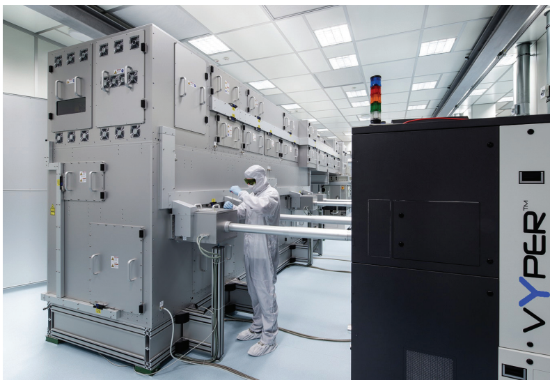
FIGURE 2. In the newest TwinVYPER system, four separate beams are combined within the system to produce a single line beam.
