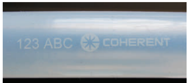
FIGURE 2. Silicon rubber tubing marked on its inner diameter with white characters.
