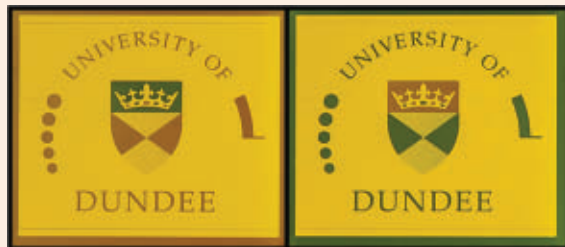
FIGURE 1. Vivid color marks created on this 25 × 25mm titanium sample using a picosecond laser. (All images courtesy of Amin Abdolvand)
