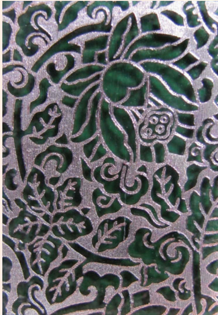
FIGURE 2. Picosecond lasers create this metallic pattern (18 × 25mm) inside clear glass.
