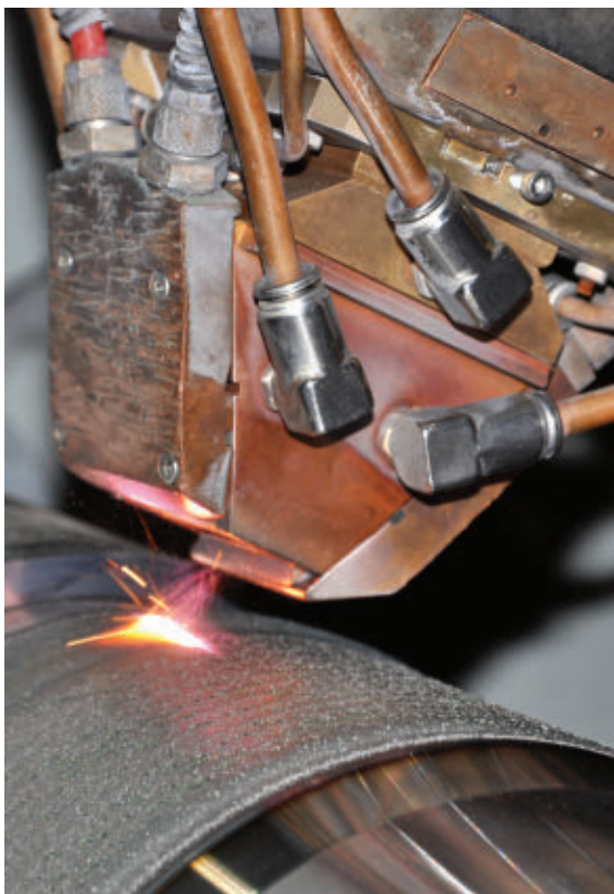
Figure 2. The output of a 4-kW direct-diode laser system (Coherent 4000L) applying a tungsten carbide blend on a seal area to provide a highly wear resistant surface.
