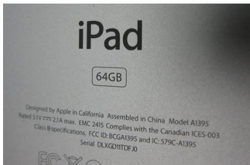
Figure 3: “Black marking” produces a high contrast, subsurface mark on anodized aluminum.
