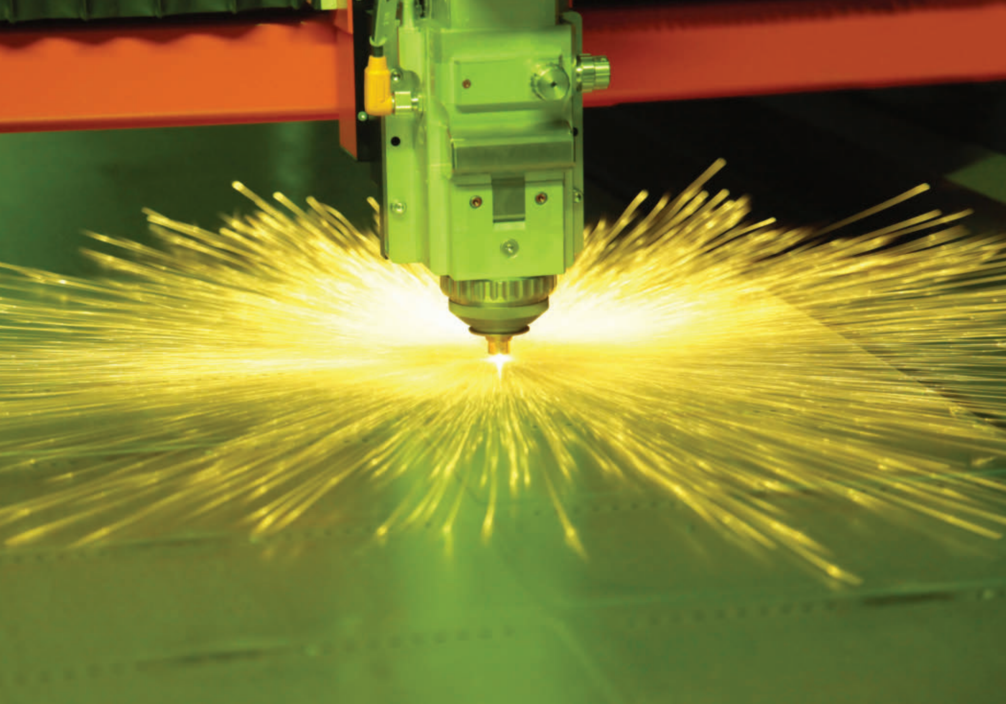
Figure 1. Different types of materials processing, such as cutting and welding metal or drilling micron-sized holes and scribing thin films, call for different types of lasers. Whatever laser is chosen to do the job, the statistical discipline of process qualification is crucial to ensuring a process can operate successfully and around the clock despite variations, such as materials, fixtures, laser output, beam delivery and ambient conditions.
