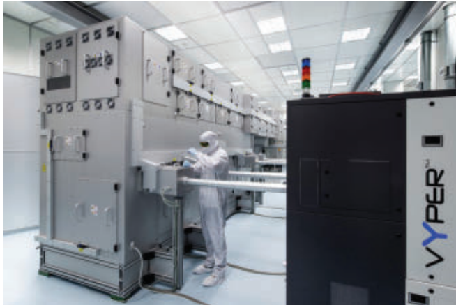
FIGURE 4. In the new Coherent LineBeam 1000/TwinVYPER system, the output from four separate lasers is combined within the system to produce a single line beam.
