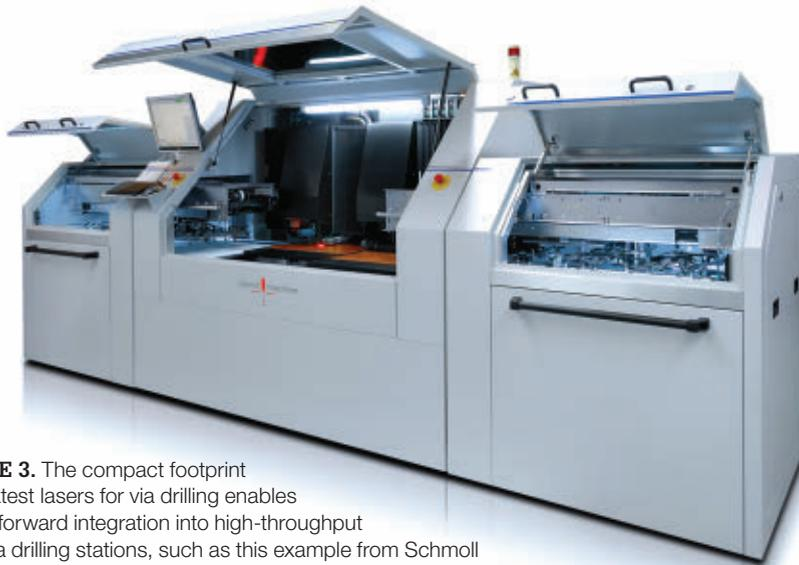
**FIGURE 3.** The compact footprint of the latest lasers for via drilling enables straightforward integration into high-throughput microvia drilling stations, such as this example from Schmolz Maschinen GmbH. (Courtesy of Schmolz Maschinen GmbH)
