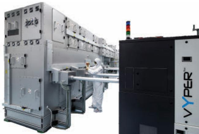
**FIGURE 2.** The evolving needs of the flat panel display market are met with a scalable Line Beam Annealing System, where multiple excimer laser beams are combined and then shaped to form a single line-shaped profile. (Courtesy of Coherent)
