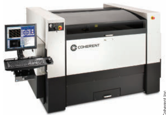
Figure 2. The Coherent Meta 2C is a compact CO 2 laser-based machine tool used at Intersign for plastics processing.
