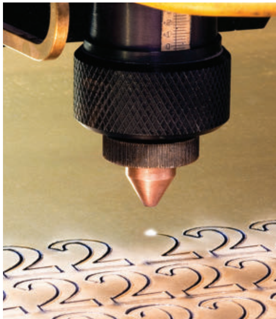
Figure 5. Laser cutting offers faster processing speeds and less postcutting processing than a router.
