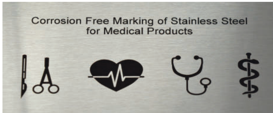
FIGURE 2. These black marks were created on 1.4301 stainless steel using a Coherent Rapid NX picosecond laser incorporated in a Rofin PowerLine marking subsystem.
