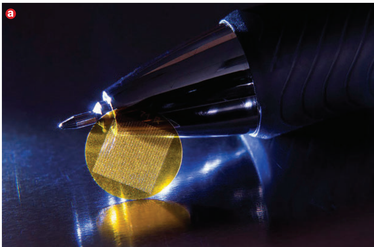
Lasers help manufacturers micromachine plastics (a) and metals (b) by drilling micron-size holes.
