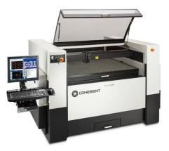
Coherent's laser cutting tool "META" has an operating range of 1.25m x 1.25m and can handle half sized medium format plates without any problem. Available laser powers range from 400 to 1000W enabling cutting of up to 3 mm of stainless steel. Employing  $CO_2$  lasers, it is also possible to cut plastics and organics with high precision.
