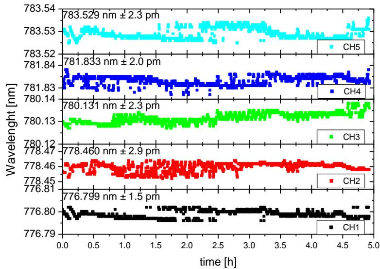
Figure 3. Wavelength switching repeatability for approximately 3600 switching events.
