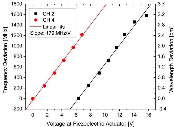
Figure 5: Individual channel fine tuning with piezoelectric actuator.
