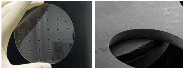
Figure 5. 3-mm-diameter (button) holes cut in a 5.5-mm-thick glass substrate.
