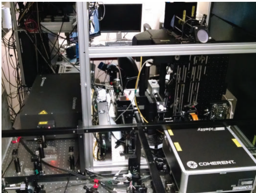
Optogenetics microscopy setup: A ytterbium fiber laser (Coherent Fidelity), which is used primarily for photoactivation, is used in conjunction with a tunable ultrafast laser (Coherent Chameleon; background). (Courtesy of Adam Packer, Häusser lab, University College London)
