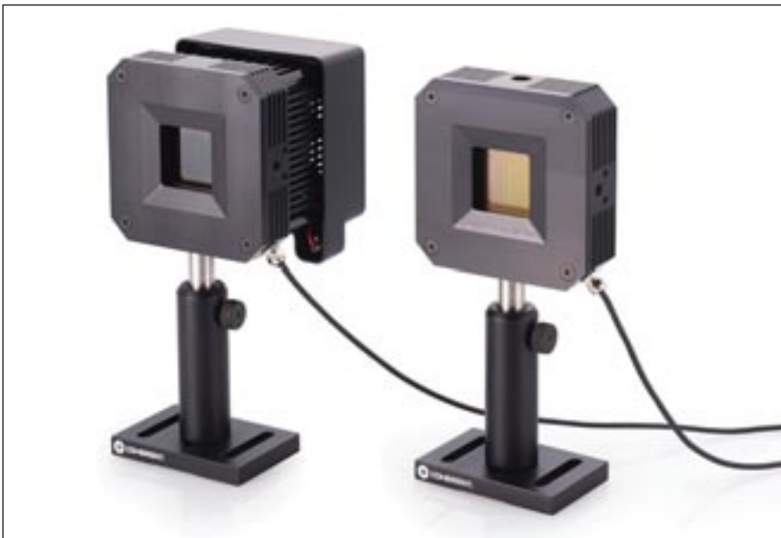
Figure 5. Thin film thermoelectric sensors are available with a broadband coating, which operates from 300 nm to 11 \mu m, and a higher damage threshold (up to 14 kW/cm 2 ) coating, which covers both 355 nm to 1100 nm and 9 \mu m to 11 \mu m.
