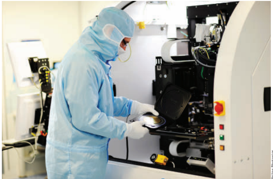
A semiconductor laser, in this case for a VCSEL (vertical-cavity surface-emitting laser), being loaded into an automated bonding machine as part of the production process.
