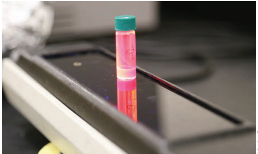
Quantum dots, like those seen in this vial, could form the basis for future semiconductor lasers, with precise control over output wavelength determined by the size of the quantum dots.
