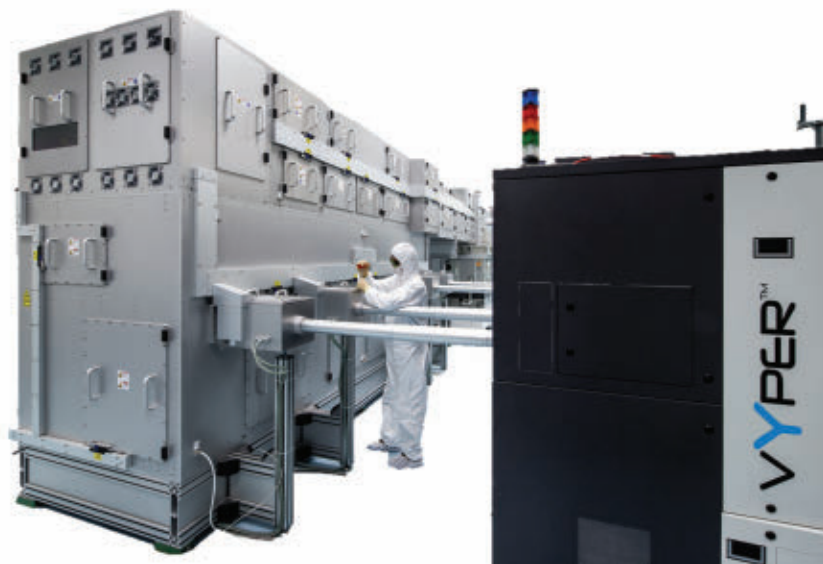
High-power scaling for large format poly-Si annealing shown here with two dual-oscillator VYPER lasers, with all four beams merging into a 1300-mm length processing beam.
