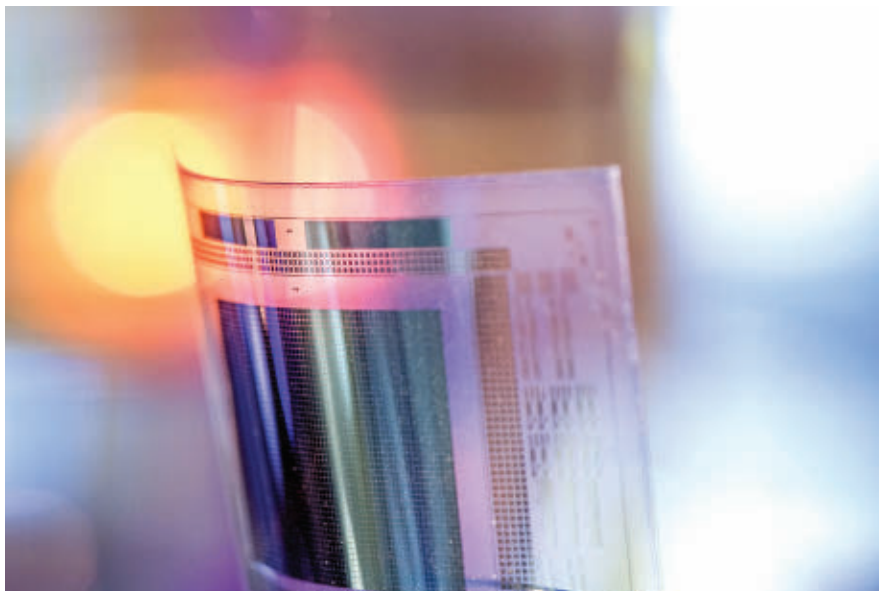
Excimer lasers enable high-volume manufacturing of flexible displays; a key step is laser lift-off where high-duty cycle excimer lasers are used to release the flexible displays from a rigid temporary carrier.
