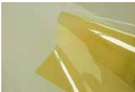
Figure 3: Polyimide coated display glass after laser lift-off separation
