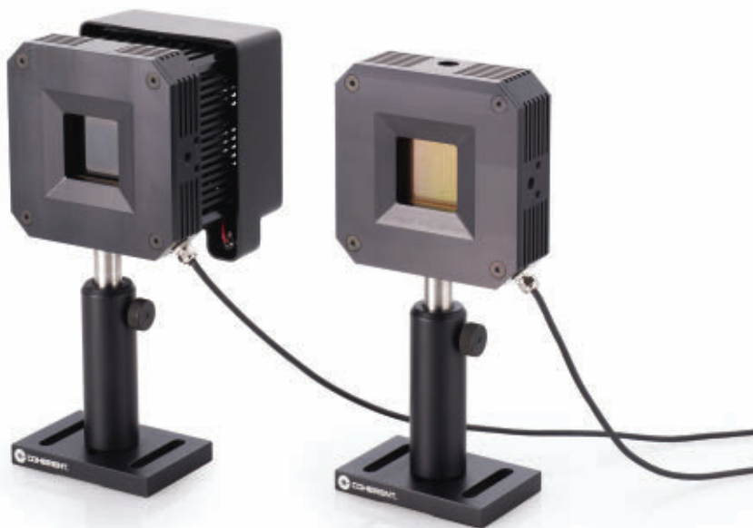
Figure 5. Thin-film thermoelectric sensors are available with a broadband coating, which operates from 300 nm to 11 \mu\text{m} , and a higher damage threshold (up to 14 \text{kW}/\text{cm}^2 ) coating, which covers both 355 to 1100 nm and 9 to 11 \mu\text{m} .
