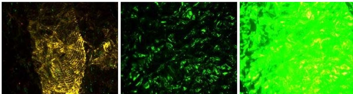
*Figure 1. One of the advantages of green (532nm) laser light is that it generates high fluorescence intensity. On this Rhodamine-dusted aluminum foil, this allows the camera aperture to be greatly reduced to obtain sufficient depth of focus for this highly contoured surface (a). This same dusted print could not be seen with an ALS (b). Even with an extended exposure time with the ALS (c).*
