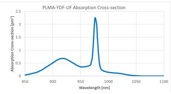
Figure 1: PLMA-YDF-UF absorption cross-section.
