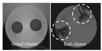
Figure 2: Example of good cleave (left) and bad cleave (right).
