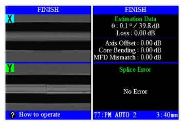
Figure 3: Optimized splice with minimal heat distortion and low loss.
