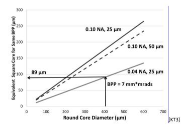
Figure 7 Plot of the equivalent square core diameter required to replace a round core diameter (for 10 meters) to achieve a flat top intensity profile while maintaining the same BPP. The core diameter for the square cores is a measurement from the flat-flat section of the square. The BPP is calculated based on the diagonal length of the square core as it's the longest length. The three lines displayed are based on the 3 different launch conditions explored.
