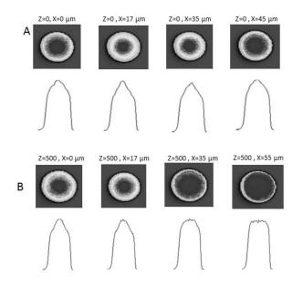
Figure 2 Near field images and intensity profiles for 200 micron core fiber misalignment experiment. (A) Misalignment in the radial direction (X-direction) only. (B) Misalignment in both the axial (Z-direction), and radial direction.
