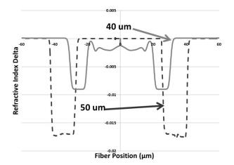
Figure 8 Comparison of the refractive index profiles of a standard 50 micron round beam delivery fiber to a 40 micron core fiber with a modified index profile designed to induce a flat-top output.
