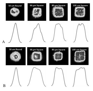
Figure 4 A) Near field image and intensity profiles for the 50 micron round core baseline fiber with the 66, 80 & 100 micron square core fibers for A) 0.04 NA launch. B) 0.10 NA launch. All samples were 10 meters in length.
