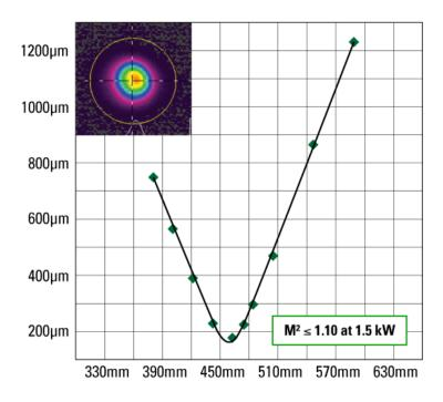
Beam quality, M2, achieved with a 0.06 NA, 25/400  $\mu$ m, Yb-fiber operating at an output power of 1500 watts. Lower NA LMA fibers deliver excellent beam quality at the highest powers.
