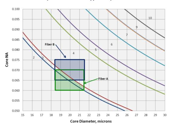
Number of linearly polarized modes supported by fibers with different core sizes and NAs operating at 1064 nm. Lower NA fiber offers the largest operating range of fewest modes making it ideally suited for high powers while maintaining beam quality and fiber reliability.
