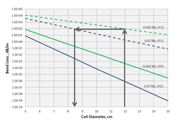
LP01 and LP11 bend losses of 20  $\mu$ m core diameter fibers at 1060 nm vs. coil diameter for 0.065 NA (in green) fiber and 0.07 NA (in blue) fiber. The 0.065 NA fiber has greater HOM bend loss enabling users to more easily discriminate the fundamental (LP01) mode from the HOMs making it easier to design fiber lasers with diffraction limited beam quality.
