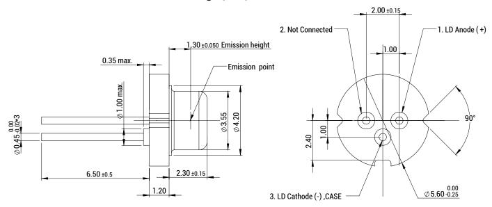
Figure 1: Technical drawing of TO-56 package including dimensions left: side view, right: bottom view, General Tolerance +/- 0.1 mm, Lead finish Au
