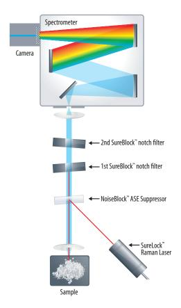
Ondax SureBlock™ Notch filters are reflective volume holographic gratings (VHGs), produced in a proprietary glass designed for long lifetime, high efficiency and excellent transmission. Ondax's fabrication process is highly stabilized to ensure excellent part-to-part repeatability.
