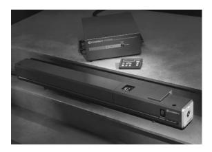
The Innova<sup>™</sup> 300C MotoFRED<sup>™</sup> ion laser utilizes intra-cavity frequency doubling in BBO crystals to produce deep-UV, CW at seven wavelengths light in the range 229-264.3 nm. This advanced small-frame system features a motorized crystal shifter and active stabilization for enhanced user-productivity. With deep-UV output powers up to 0.2W, the 300C MotoFRED is ideal for moderate volume manufacturing and advanced research applications.
