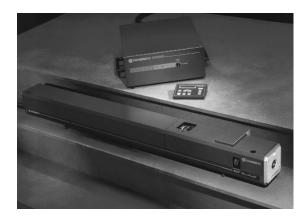
The Innova® 90C FRED™ ion laser utilizes intra-cavity frequency doubling in BBO crystals to produce deep-UV, CW light at seven wavelengths in the range 229-264.3 nm. This small-frame ion laser provides output power up to 0.1W and is an ideal basic system for laboratory use.
