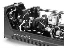
The Innova® Sabre® MotoFreD™ ion laser utilizes intra-cavity frequency doubling in BBO crystals to produce deep-UV, CW light at several wavelengths in the range 229-264.3 nm. In addition to a motorized crystal shifter, the system offers the most comprehensive range of automation and stabilization features, combined with specified output powers up to 1W, for highvolume manufacturing applications.
