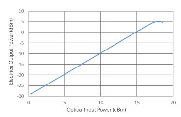
RF output power as a function of the optical input power for a bias voltage of 4 V at a frequency of 20 GHz
