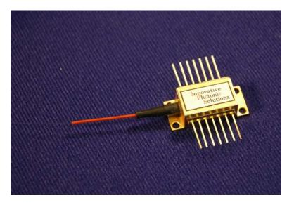
Figure 9. Fiber coupled HECL in a 14-Pin butterfly package
