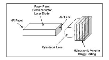
Figure 1. Hybrid ECL/DBR Laser (HECL)
