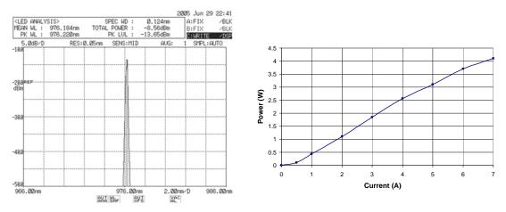
Figure 8. Spectral Plot and LI Curve of High Power/High Spectral Brightness 976 nm Spectrum Stabilized Laser
