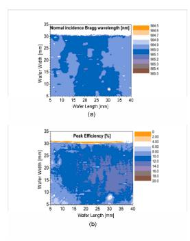
Figure 4. VHG wafer testing: 250 µm resolution measurement across 30 x 40 mm wafer. (a) map of normal incidence Bragg wavelength. (b) Map of peak diffraction efficiency
