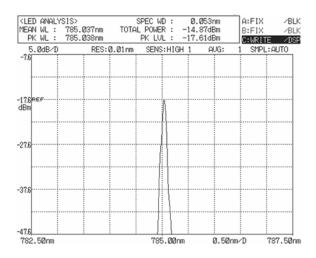
Figure 7. Spectral Plot of Ultra-Narrow Spectrum Stabilized 785 nm Multi-Mode Laser Designed for High Resolution Raman Spectroscopy Applications
